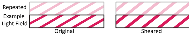
Figure 7: For a simple planar pattern, the discontinuities in the original light field can be removed by applying a horizontal shear.
