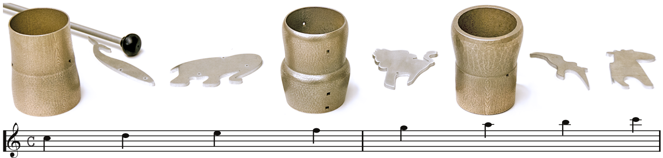
Figure 1: Customized instrument. A set of optimized 2D water jet cut animals and 3D printed cups form a musical scale. Provided with a user-supplied 3D shape and target sound characteristics of the desired frequencies and their amplitudes, our method optimizes the geometry of the object to realize the desired sound (see video).
