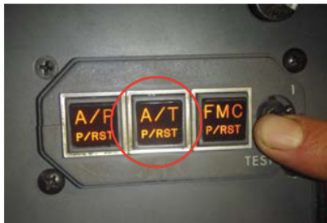
Figure D- 9. Flashing amber A/T P/RST (Department for Transport/Air Accidents Investigation Branch, 2009)
