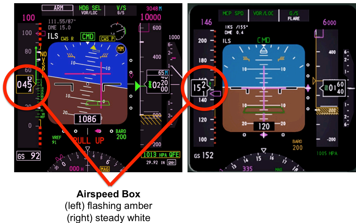
Figure 4-6. Example of flashing airspeed box on a B737 PFD [adapted from (pmFlight, 2014)]
