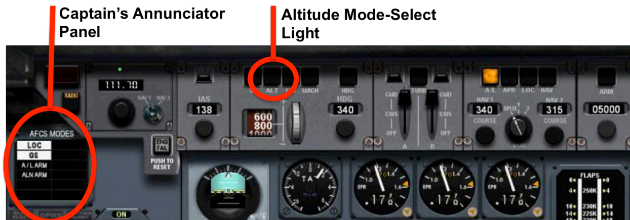
Figure 4-23. Depiction of captain's annunciator panel and altitude mode-select light in the L1011 [adapted from ("L1011 Main Panel Features," 2010)]
