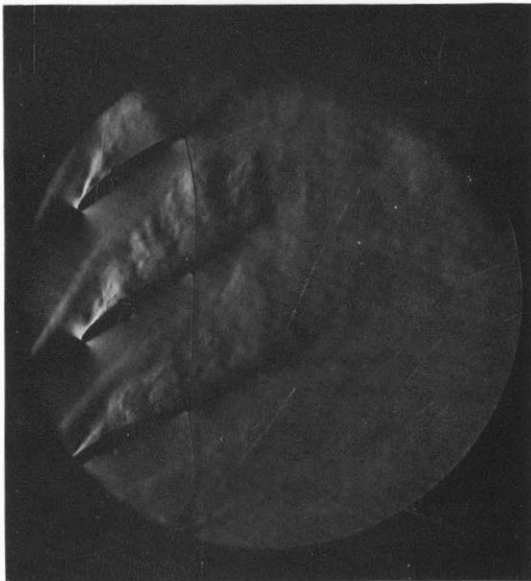
Figure 16. Spark Schlieren Photograph All Blades Stalled
