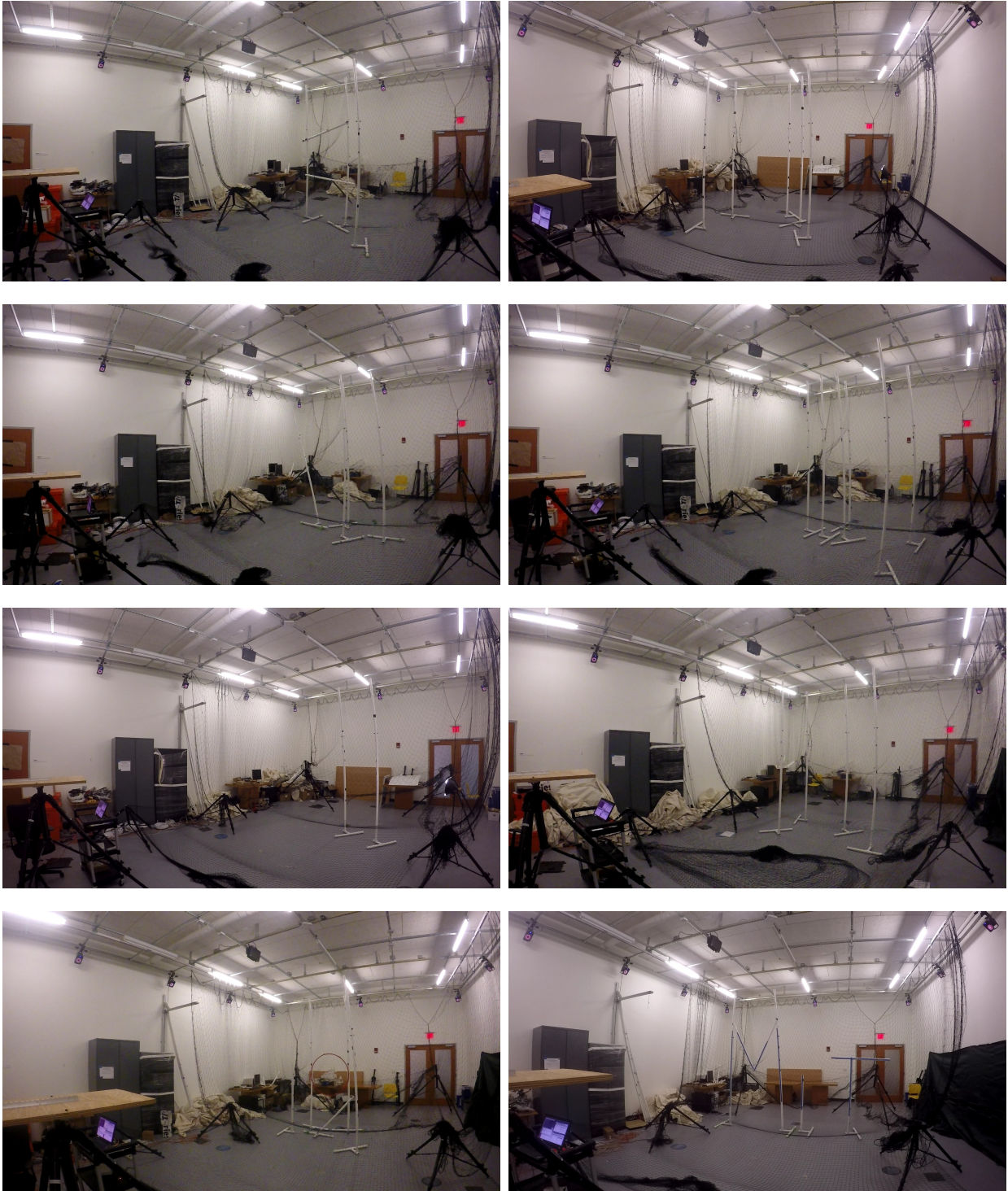
Figure 8-5: Environments 1-8 on which the online planning algorithm was tested. The obstacles include poles of different lengths in varying orientations and also a hoop of diameter equal to 0.9 m.
