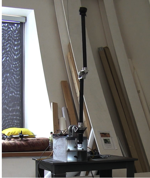
Figure 9-4: Picture of the Acrobot balancing in the upright configuration using the controller designed with SDSOS programming. A video of the controller in action is available online at https://www.youtube.com/watch?v=FeCwtvrD76L .
