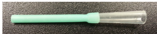
FIGURE 13. STRUCTURE OF NOZZLES USED THROUGHOUT EXPERIMENTAL TESTING. COMPLIANT SECTION HAS AN INNER DIAMETER OF 2mm WITH A WALL THICKNESS OF 0.25mm. THE DIFFUSER HAS A 2mm DIAMETER INLET, A HALF ANGLE OF 2.5 DEGREES, AND AN INLET TO OULET AREA RATIO OF 3.
