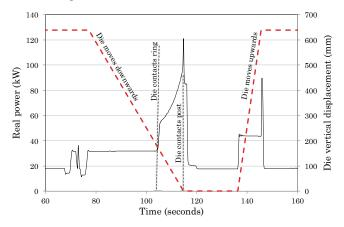
Figure 6: Power profile and die displacement for hydraulic press
