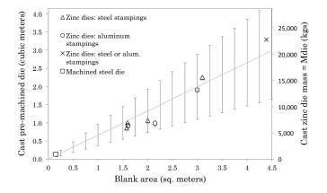
Figure 15: Blank area vs. die size. Error bars: ±45% of mass
