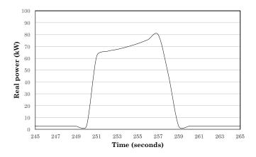
Figure 8: Forming of one part using mechanical press
