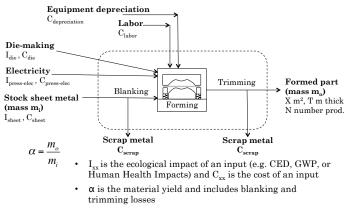
Figure 10: The ecological impacts (I<sub>xx</sub>) and costs (C<sub>xx</sub>) of forming sheet metal parts
