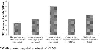
\*\*With a casting efficiency of 0.05 therm /kg
