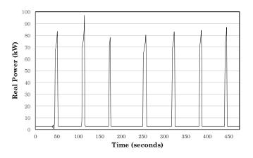
Figure 7: Power profile for forming of seven parts on the mechanical press
