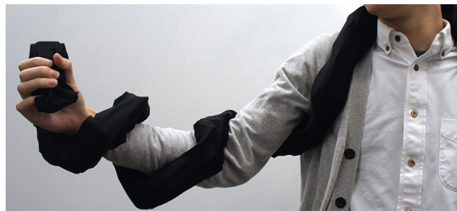
Figure 9. LineFORM wrapped around an arm to constrain body motion.
