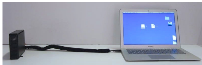
Figure 8. A shape-changing cord represents data flow through physical motion.
