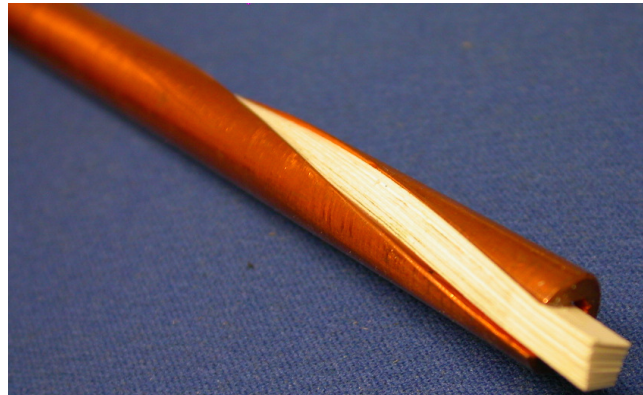
Fig. 18. Vertical stack in helical groove where the tape surfaces are parallel to the side wall of the groove.
