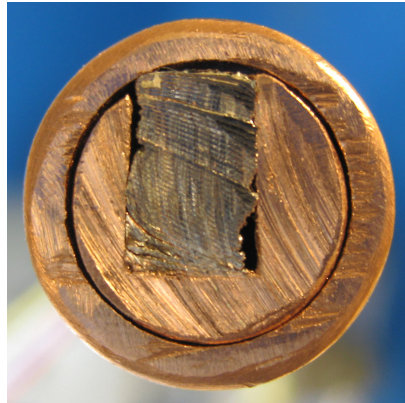
Fig. 17. Stacked-tapes distorted by twisting in helical groove of former.
