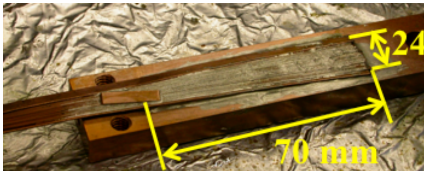
Fig. 15 A soldered folding-fan termination fabricated.
