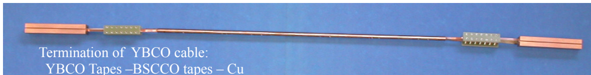
Fig. 1. 40-Tape TSTC conductor of 1.16 m long, 200 mm twist-pitch cable in 9.5 mm OD solder-filled Cu tube with REBCO-BSCCO terminations fabricated at MIT, and tested using the FBI facility at KIT, Germany.
