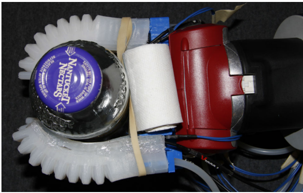
Fig. 12 The DRL soft hand with stiff backdrop inserted for object identification grasps
