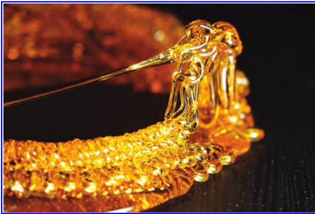
FIG. 7. Object printed with 50 mm Z-offset of the nozzle showing fluid mechanical sewing machine behavior.
