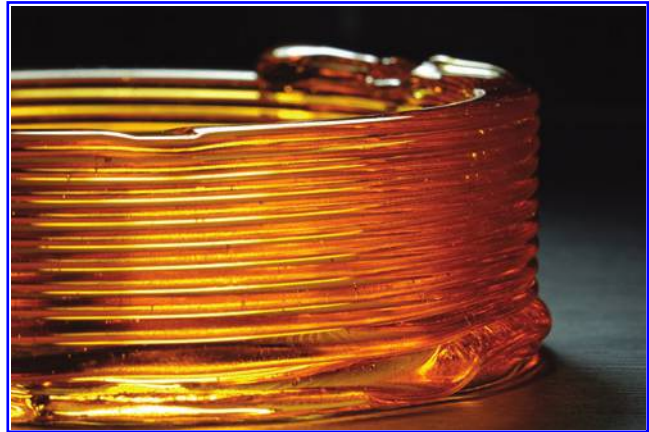
FIG. 5. Cylindrical object printed by molten sugar showing consistent extrusion result.
