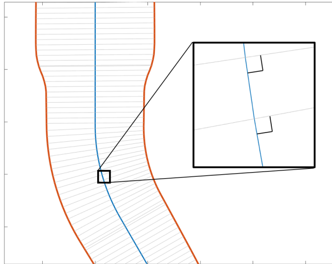
Figure 18. Contour generated by applying the half-width functions orthogonal to an RNAV procedure centerline
