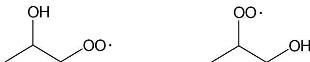
Figure 5-8: The two \beta -hydroxypropylperoxy radicals formed in the atmospheric oxidation of propene.
