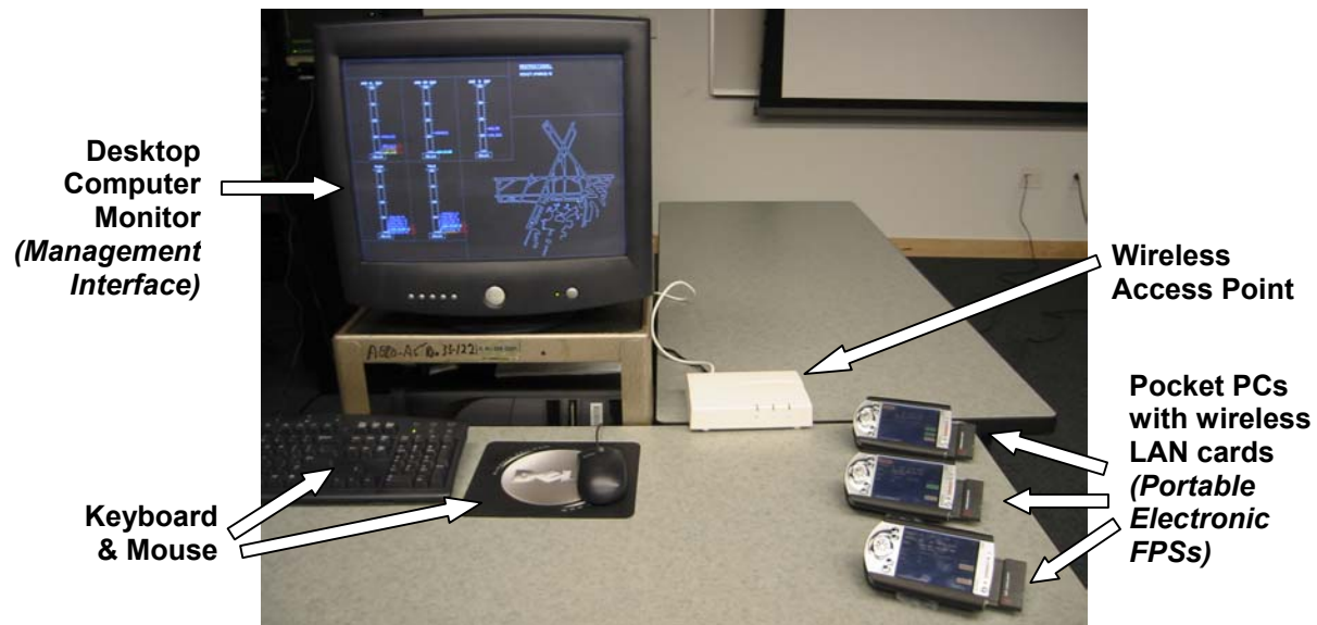
Figure 3.4: Prototype Hardware for Portable Electronic FPS System
