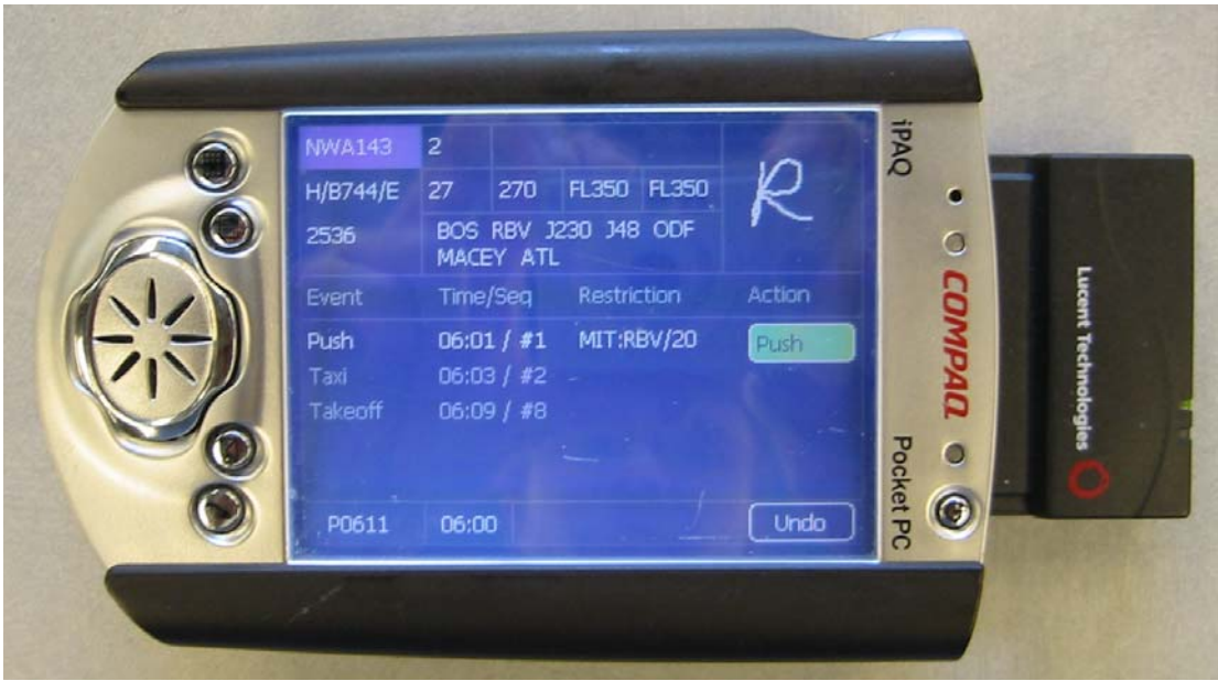
Figure 3.11: Photograph of Portable Electronic FPS Software on Pocket PC
