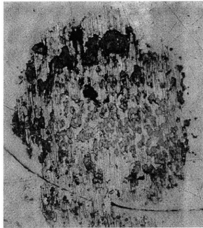
Figure A-4: Scar on one of the Ti-6Al-4V STO pads used on specimen # 3
