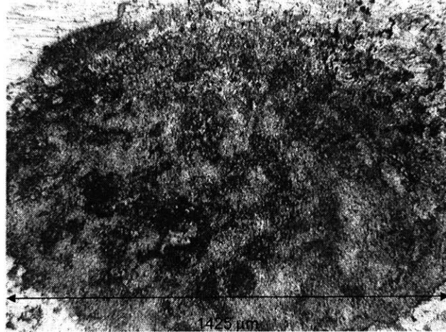
Figure 3-14: Scar obtained for P=50 N, Q\sim 37 N, and a maximal axial stress over 600 MPa (stress ratio=0.1); the contact diameter predicted by Hertz theory is close to 400\ \mu\text{m}
