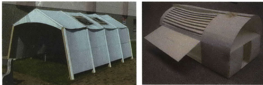
Figure 2.12. Model and first prototype of a printed paper school-house or emergency relief shelter. Pappu, Griffith, SCA, 2000.
