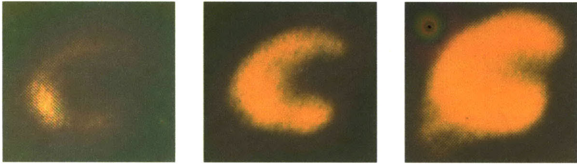
Figure 6.3 Increasing exposure times of raw (unimaged) incident beam on a film of silver nanocrystals demonstrating spatial distribution of energy within the beam.
