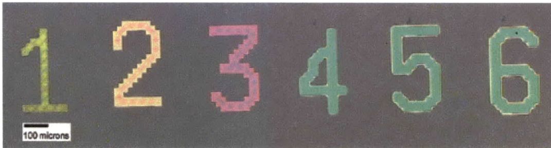
Figure 5.12. Test exposure matrix. Exposure conditions as in table 5.1.
