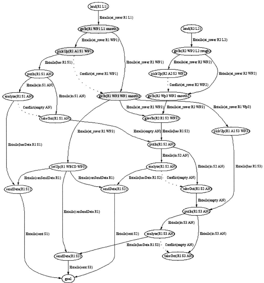
Figure 5.2. The activities “pickUp(R1 A1 S1 WP1)” and “goTo(R1 WP3 WP1)” are also affected by the changed condition through causal links from the activity “goTo(R1 WP1 L)”.
