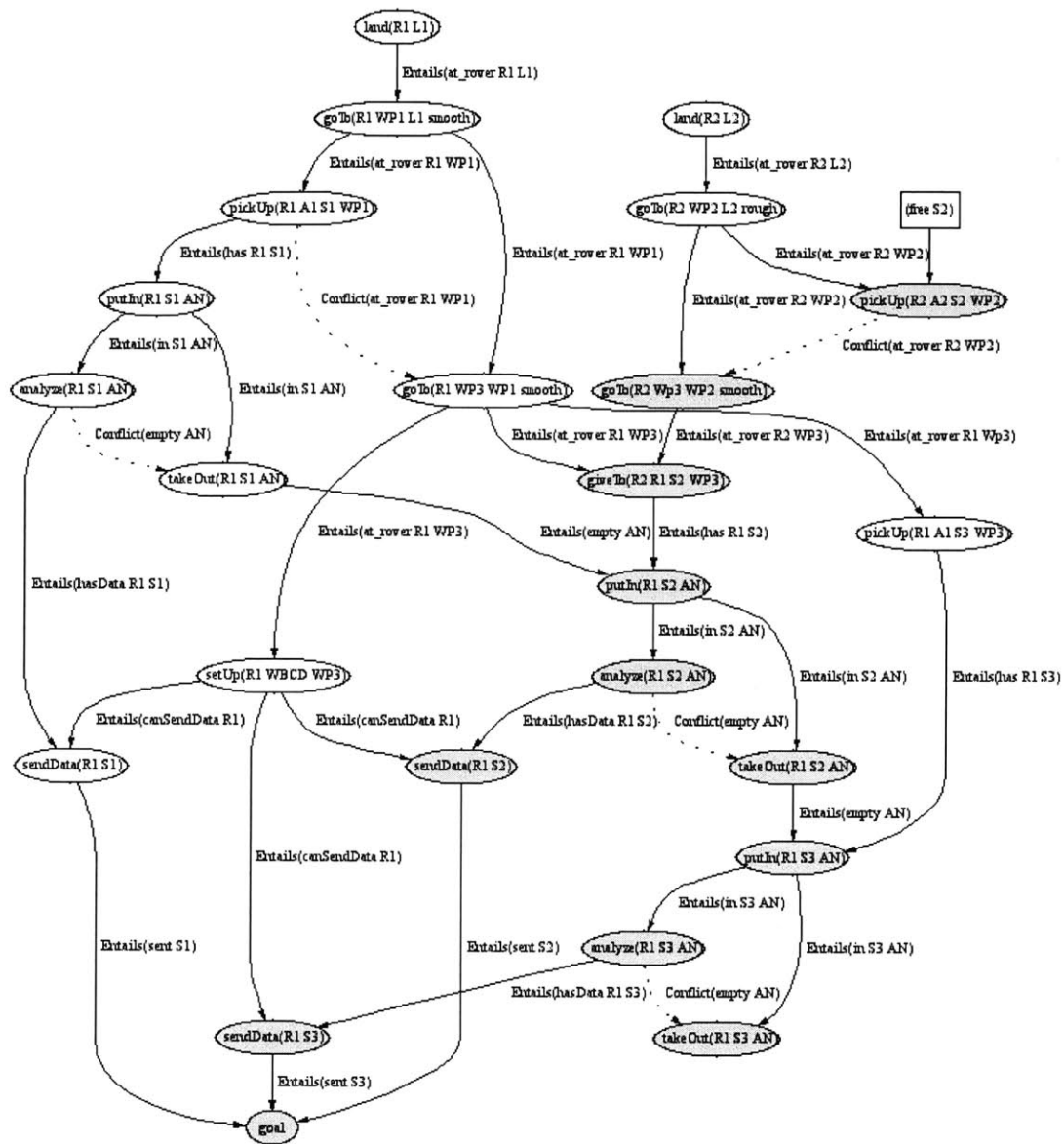
Figure 6.1. The shaded activities represent the broken subplan as a result of the changed condition “not(free S2)” which is represented by a rectangular node in the top right hand corner.
