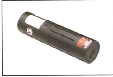
Figure 2-3: Photograph of the diode laser. This is the radiation source used in the ZPAL prototype built during the course of this research. This laser diode has a central wavelength of 400 nm and a output power of 25 mW. This laser module was manufactured by Power Technology, Inc [5].
