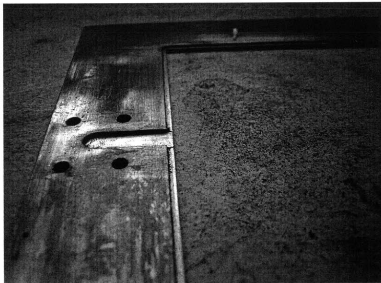
Figure 3-7: A close view of the groove cut on the bottom plate. The groove allows air to be drawn out from between the mask and wafer.
