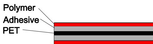
Figure 5.3: PPy / polyurethane / PET / polyurethane / PPy trilayer construction. Typical thickness for the layers are: polymer (PPy) = 10-20 \mu\text{m} , PET = 25 \mu\text{m} , Adhesive = 25-50 \mu\text{m} .
