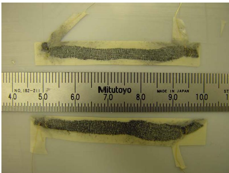
Figure C.2: Photograph of two polypyrrole coated Lycra strips encapsulated in a polyurethane. The tabs emerging to the sides are where the electrical contact is made to the strip with gold wires. The ruler is marked in mm.
