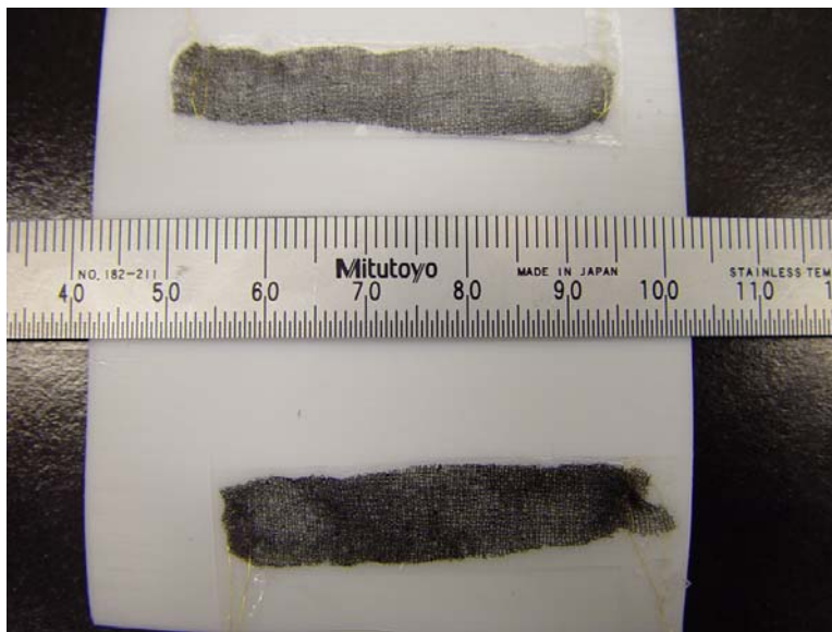
Figure C.1: Photograph of two polypyrrole coated lycra strips encapsulated in silicone. The silicone is nearly transparent and has been trimmed to be slightly larger than the coated Lycra strips. The ruler is marked in mm.
