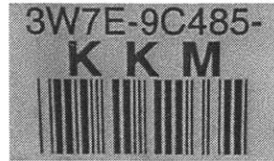
Figure 5. Part number on a Ford emission decal. Ford has recently implemented a machine readable bar code of the suffix with an eye toward implementing bar code readers at the assembly plants to improve installation accuracy.
