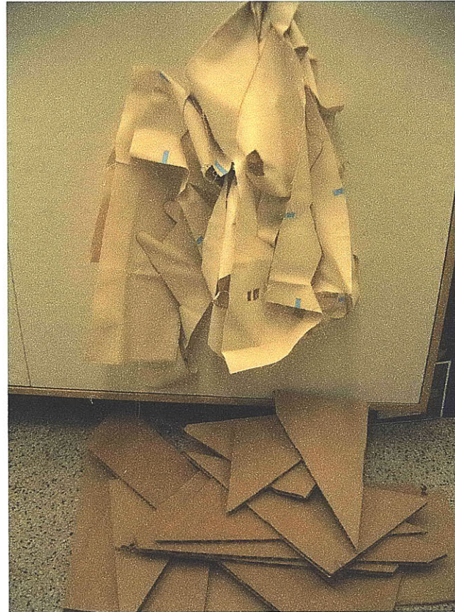
1/8" thick, birch-faced plywood was cut in a single pass. Though cut-lines were prepared for laser cutting by nesting, a lot of material was wasted.
