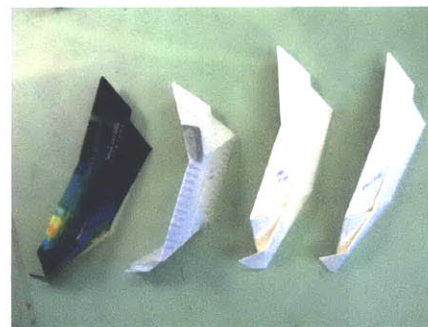
Modular belts of different thicknesses were folded to test YUPO's flexibility.
