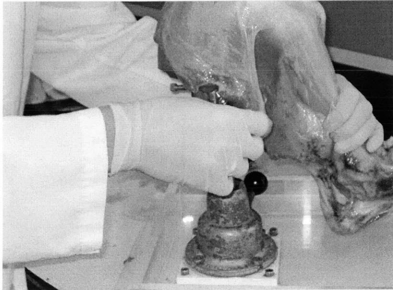
Figure 2A: Joint being secured in holder.
