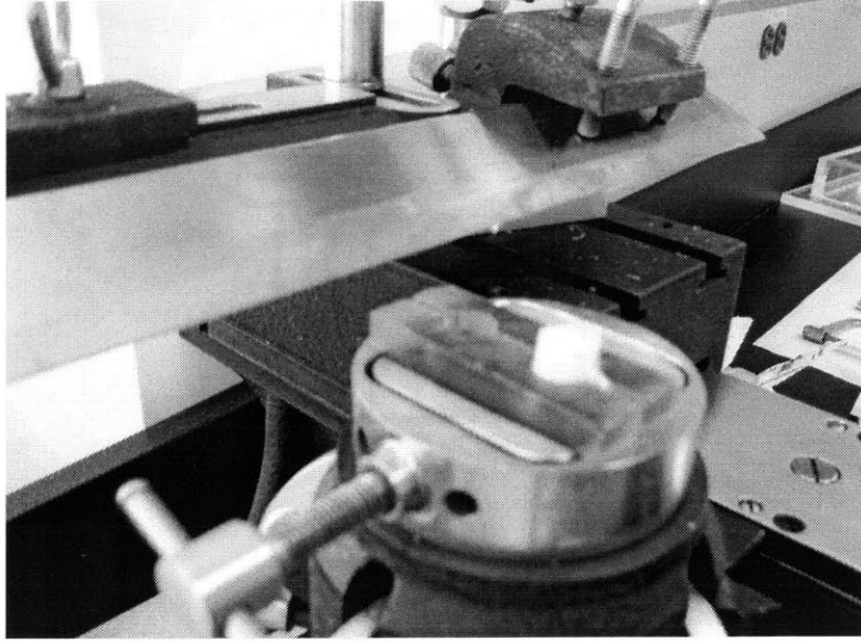
Figure 4F: Holder with core placed in the microtome and ready to be sliced.
