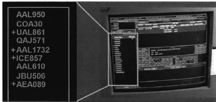
Figure 3-18: Communication window contains a list of aircraft within the sector. Aircraft equipped with Datalink have a “+” next to their aircraft ID. Controllers click on any aircraft ID to send an electronic message.
