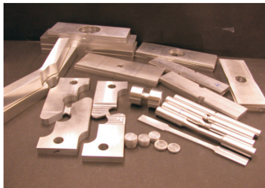
Fig. 6-1: Specimens used to calibrate the BW's fracture criterion. Courtesy Y. Bao.
