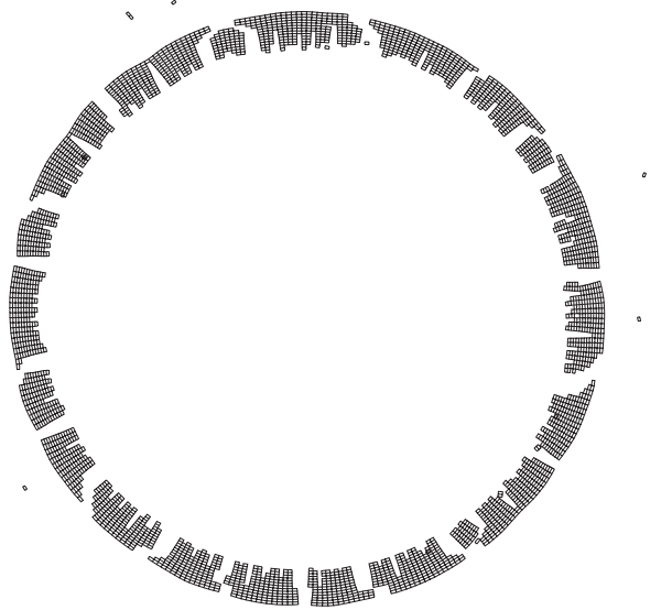
Fig. 3-3: Fragmentation of a ring under explosive loading.
