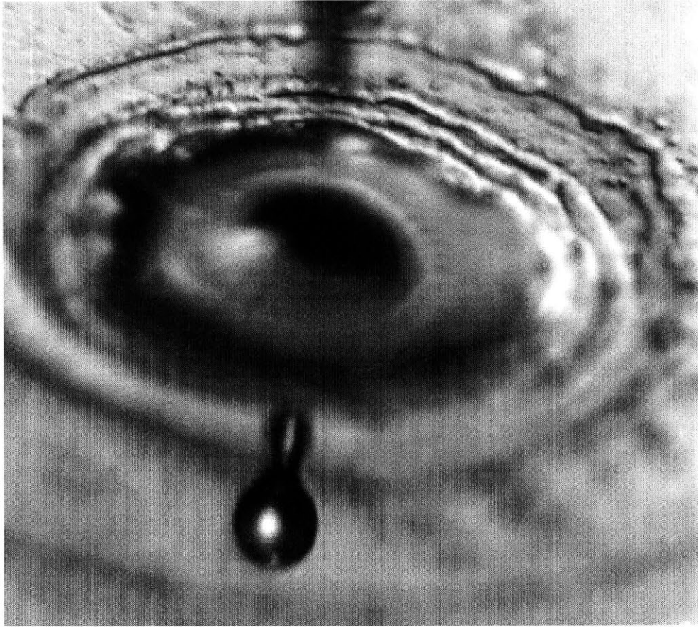
Figure 3. PAA buildup. Drop ejection with PAA binder on a standard negative pressure 40 micrometer ruby orifice builds up PAA rings around the orifice, and drop breakoff changes dramatically. Eventually, drops stop forming altogether.
