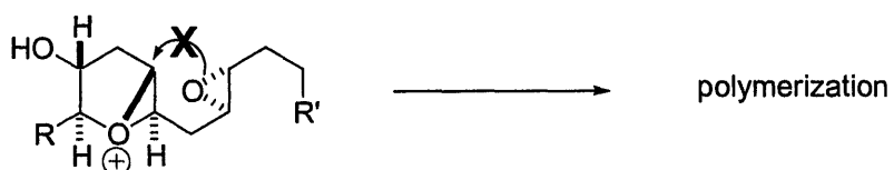
Figure 14. If a disubstituted epoxide does not act as a nucleophile polymerization may result.
