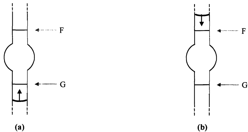
Figure 4.2. Schematic of the Ubbelohde viscometer test-section. The blue arc and arrow indicate the location of the fluid free surface and its direction of motion, respectively, while (a) filling and (b) draining.
