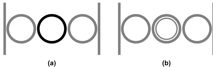
Fig. 9.1 Frequency matching strategies. (a) The SEBL dose of the middle ring is increased to precisely widen the middle-ring waveguide. (b) A secondary non-resonant ring is introduced at the center of the middle ring to increase the effective index of the middle ring-waveguide. Both methods lower the resonant frequency of the middle ring to match it to the outer rings. (a) is particularly useful if a maskless lithography technique such as SEBL is used and can be applied in either mask manufacturing or direct device writing. (b) is particularly useful for photolithography or nano-imprint lithography when little control is exerted on the mask manufacturing process.
