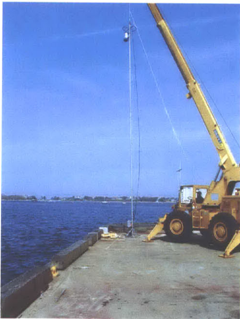
Figure 12: The transducers mounted on a 10m pole.
