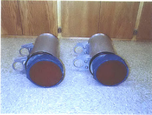
Figure 11: Transducers with pressure housing.
