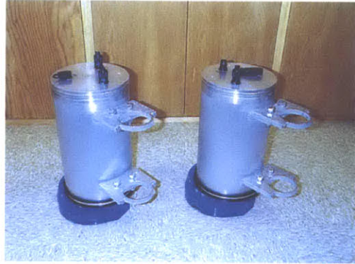
Figure 11: Transducers with pressure housing.
