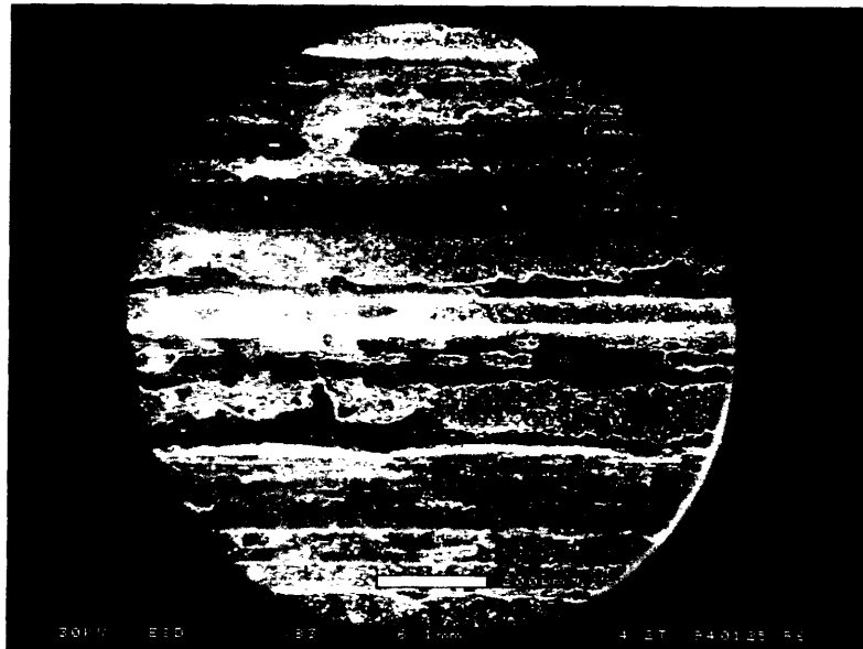
Figure 4.19 Sever plowing of a smooth copper shaft tested in vacuum of 1.3 \times 10^{-4} Pa at 245 °C. Normal Load= 2.5 N
