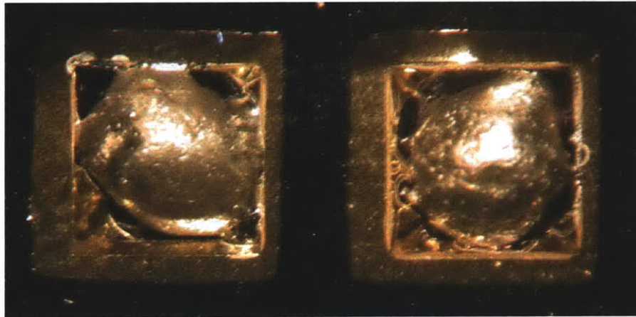
Figure 6-16. Gold-Tin Seal-Off with Extended Outgassing
