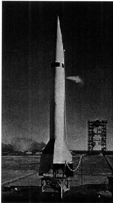
Figure 12: MX-774 Test Missile. Nicknamed "The Old Fashioned" for its visual and technical resemblance to the V2 rocket. Courtesy, Astronautix.com
