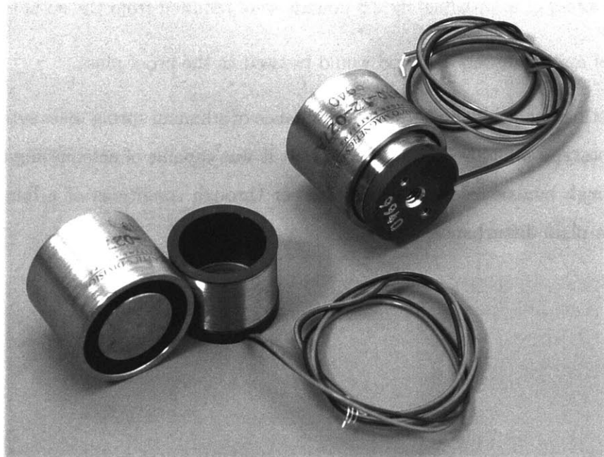
Figure 2-7: Photograph of BEI LA10-12-027A voice coil assembly, single core assembly, and single coil assembly.
