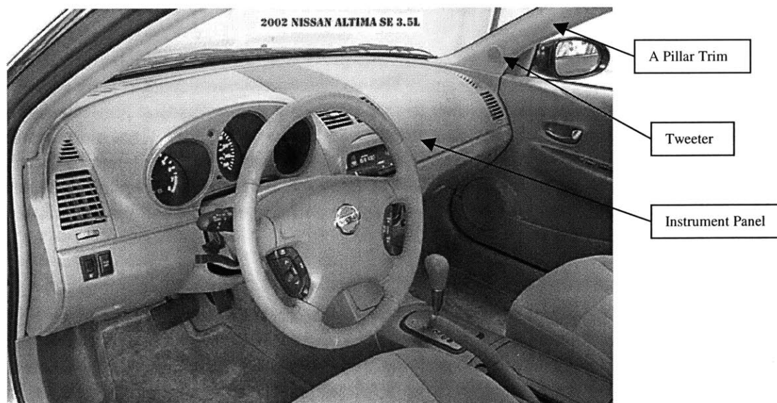
Figure 9 –Illustration and Location of 2002 Nissan Altima Tweeter and Associated Parts
