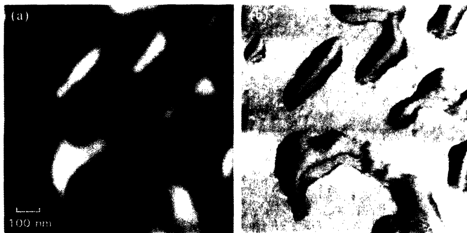
Figure 4-8: AFM scans of a \text{SnO}_2 thin film after 20 Å thick BCP deposition: (a) height and (b) phase.
