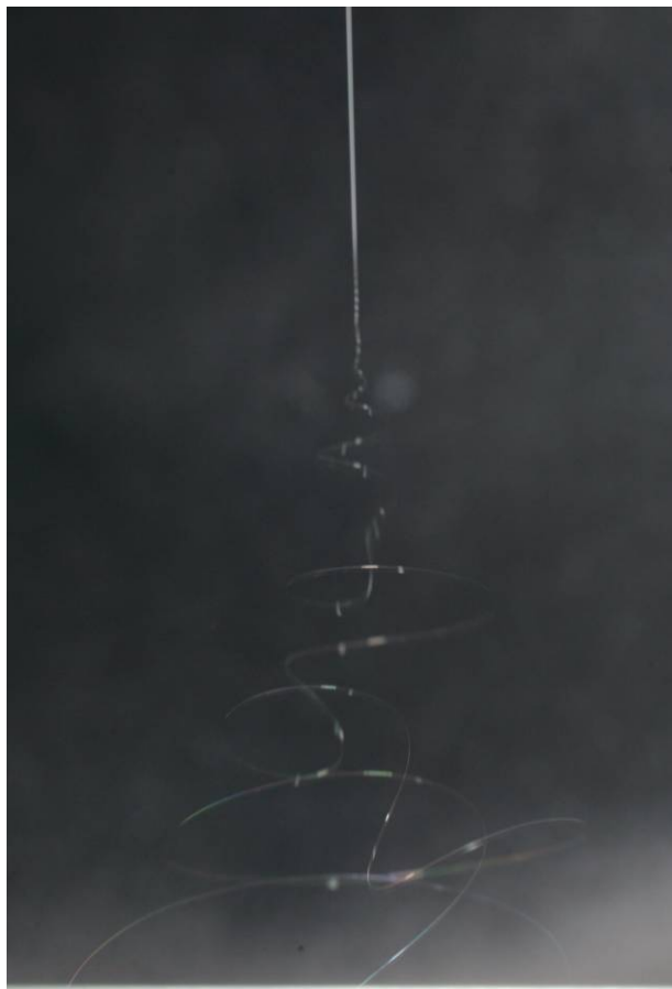
Figure 11: A view of the whipping instability when electrospinning poly(ethylene oxide). The electrospinning conditions included a 10 kV nozzle voltage, 170 mm electrode separation, 2% (w/w) polymer solution in distilled water, 2 \times 10^6 molecular weight, and 0.5 mL/hr flow.
