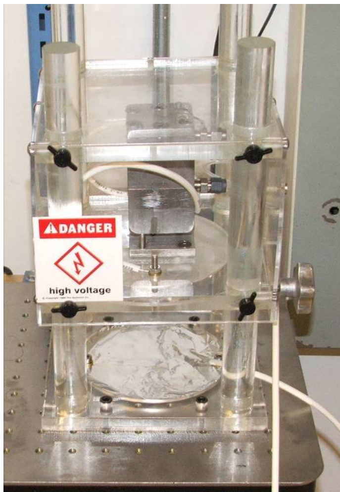
Figure 13: Photograph of completed electrospinner. The clear plastic parts are all made from poly(methyl methacrylate), and the nozzle assembly from Figure 12 is visible in the center of the photo.
