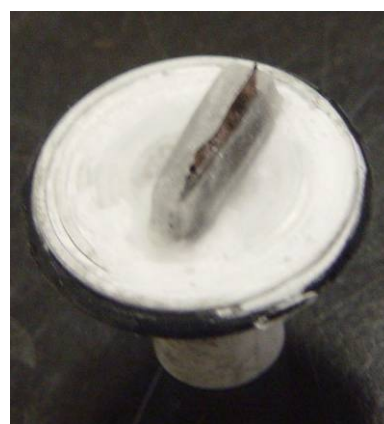
Figure 5: Mounted ice block with embedded polypyrrole film.
