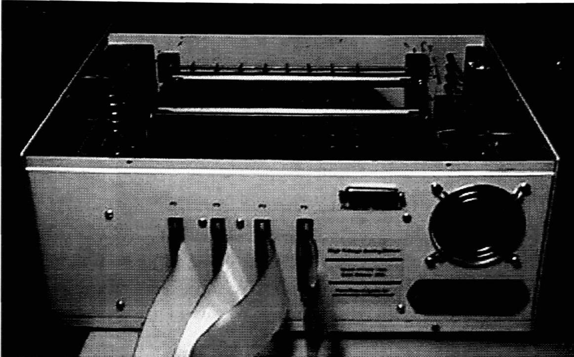
Figure 10. Back view of the HVADI, showing connections for the 4 ribbon cables and the parallel port.
