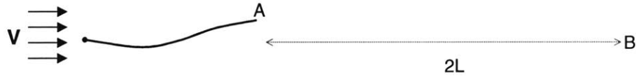
Figure 6-31: Depiction of sample points for frequency analysis of the flapping body. Point A is the trailing edge of the body, whose cross-stream displacement is used for analysis, while point B is at the centerline of the wake, two body lengths downstream of the trailing edge equilibrium position, where the cross-stream flow velocity is used for analysis.
