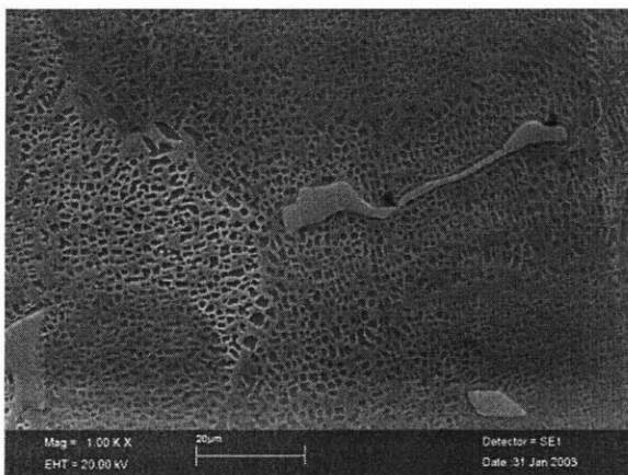
Figure 10 - Grain boundary carbides in after-service material
