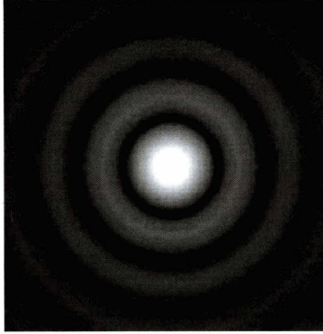
Figure 3.2 Airy Disk with Outer Rings Digitally Enhanced to Make More Easily Visible [49]
