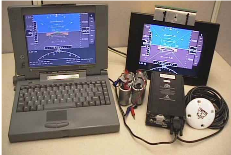
Figure 6.6: Portable Configuration Flight Test System with Repeater Display
