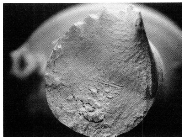
FIGURE 59 - Photomicrographs of Fracture Surfaces of GMA HAZ Specimens for Free Corrosion (top, 86 X), Cathodically Protected (middle, 45 X) and Hydrogen Generating (bottom, 36 X) Showing Effect of Strain Rate (Strain Rate .00000833/sec).
