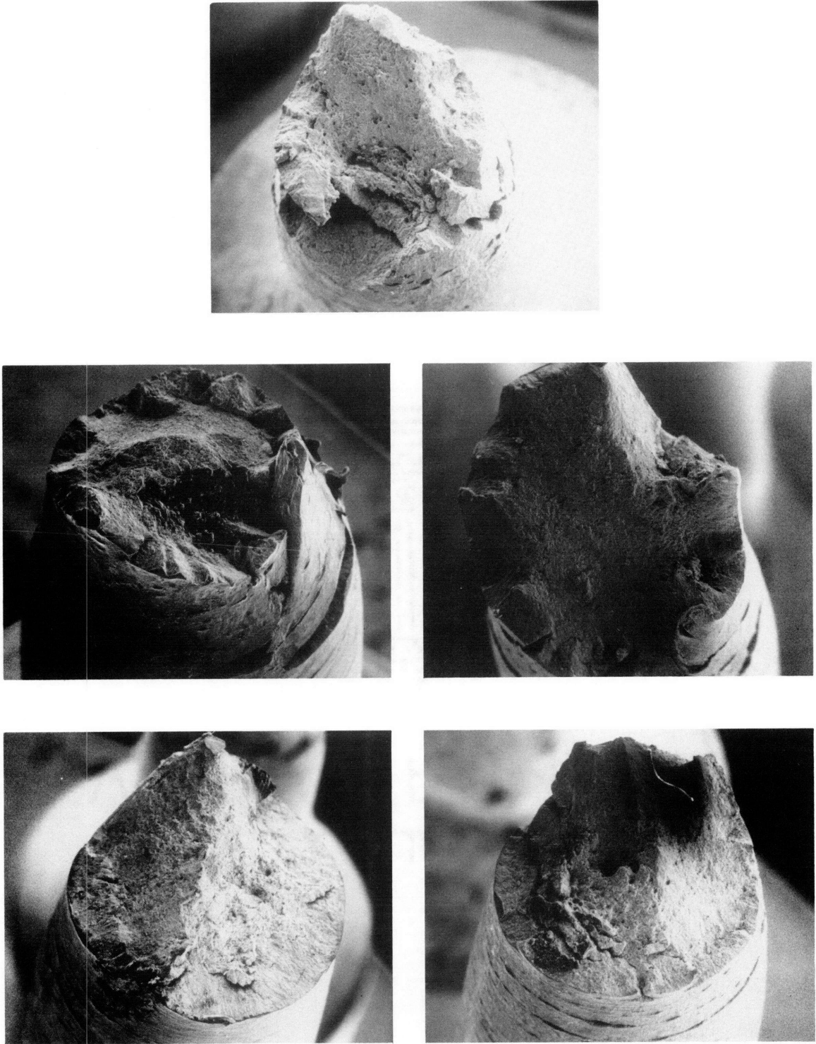
FIGURE 60 - Photomicrographs of Fracture Surfaces of Base Metal (top), GMA Weld Metal (middle left), GMA HAZ (middle right), SAW Weld Metal (bottom left) and SAW HAZ (bottom right) Showing Effect of Material (25 X). Strain Rate .0000667/sec, Applied Potential -1250 mv SCE.
