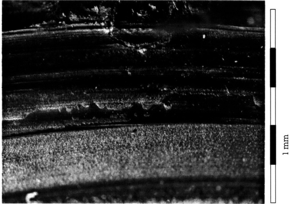
Figure 23: The top of the CC#1 seal. Worn with mud for 1.06 million cycles. Magnification 17x. The measurements for this run are shown in Fig. 28.
