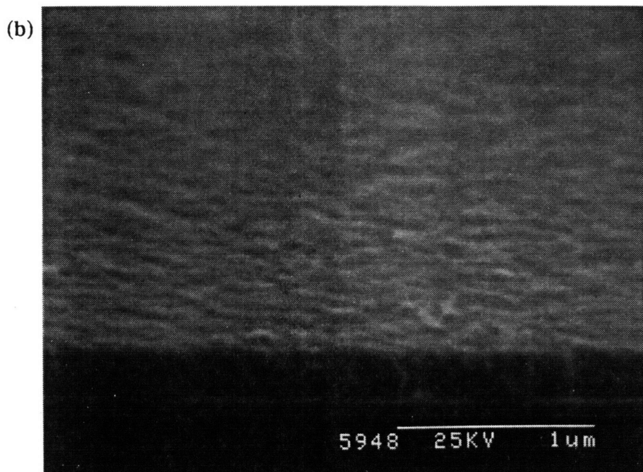
Figure 6.19 SEM micrographs of MgO films described in Figure 6.18 grown on: (a) ion milled \text{LaAlO}_3 substrate, and (b) annealed, ion milled \text{LaAlO}_3 substrate.
