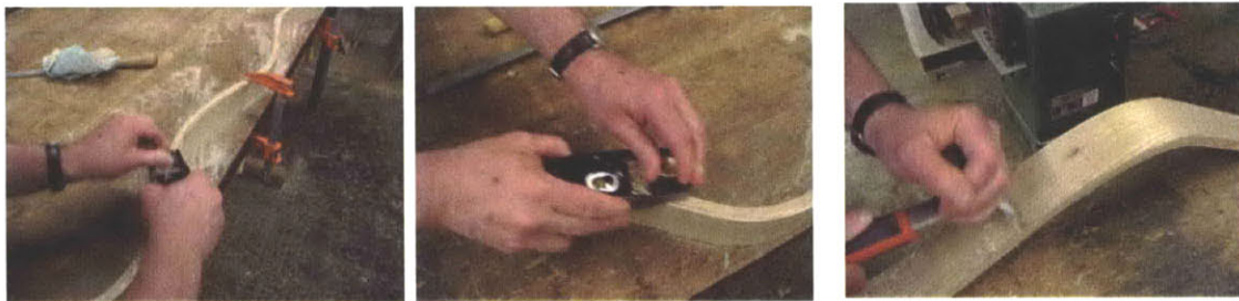
Figure 5.1.5b Once the bent structure is separated from the mold, we use hand tools to clean and smoothen the surface. In our case, we used a handsaw to cut out another shape from the bent piece of wood.
