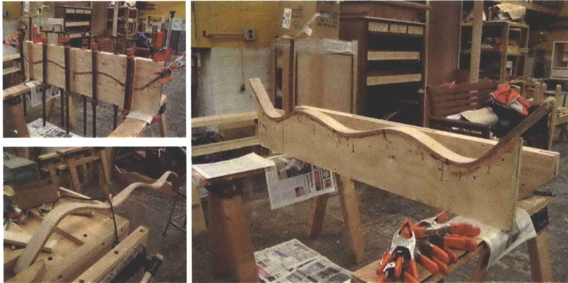
Figure 5.1.5a Bent lamination using 8 layers of Ash.
