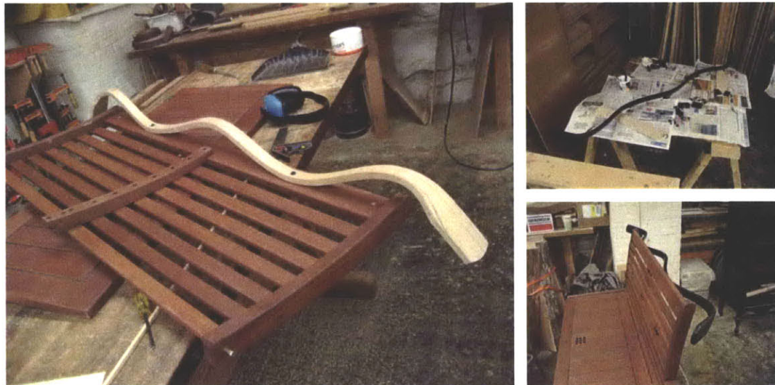
Figure 5.1.5c Bolt structures are made to de/attach the arm structure to the bench. Afterwards, India black dye is applied followed by coats of satin varnish for a clean look before attaching it to the back of the bench
