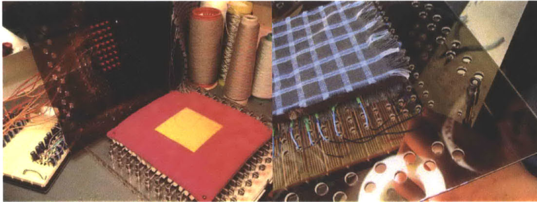
Figure 4.1.8 TechStyle: an I/O e-Fabric From left to right: floating conductive fibers successfully signal coordinate points for output mode; input and output mode is incorporated in the structure of a woven fabric piece.
