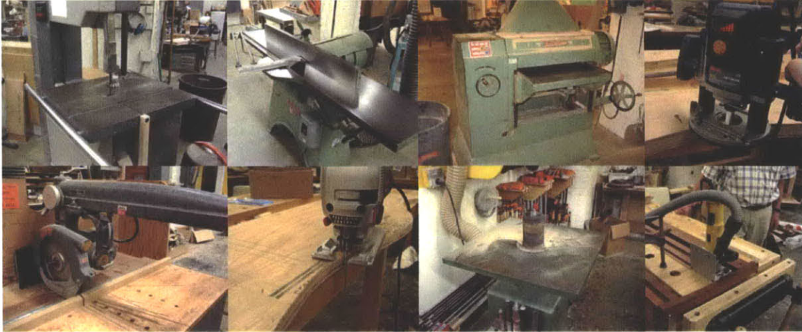
Figure 5.1.4 Woodshop tools used to make the Audio Time-Lapse Bench Tools include: band saw, jointer, planer, hand tools-saw, drill, router, sander, and the drill press.
