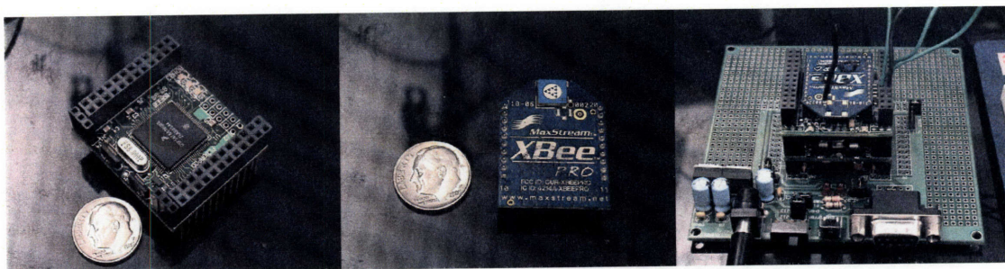
Figure 5-10: Plugapod TM microcontroller chip (left), ZigBee TM wireless components (center), and board assembly (right) used to control prototypes.
