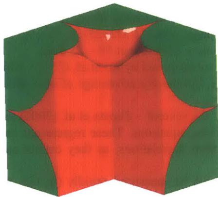
Fig.2.5.a. Bulk water at air entry
