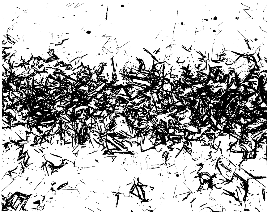
Figure 9. 24Ni3Mn Alloy, having a grain size of 0.025 mm, reacted at -115^{\circ}\text{C} to 1 percent transformation. Note a long dense cluster. Etched with 25 percent Sodium Bisulphite in water. 200X.
