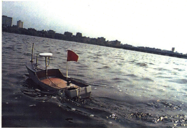
Figure 19 Experimental Setup. Frame 1: Control software being downloaded into ARTEMIS before tether is detached. Frame 2: After tether is detached, ARTEMIS is launched (it is light enough that two persons can carry it). Frame 3: ARTEMIS under way performing automated bathymetry.
