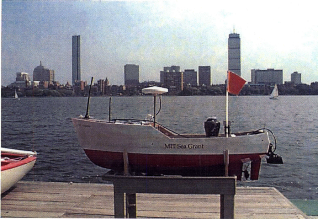
Figure 2 The 1.4-meter-long Autonomous Surface Craft (ASC) ARTEMIS configured for automated bathymetry mapping. ARTEMIS is equipped with a microcomputer for autonomous guidance, a GPS system for navigation, a depth sounder for bathymetric-data-collection, and a radio modem for data transmission in real-time.
